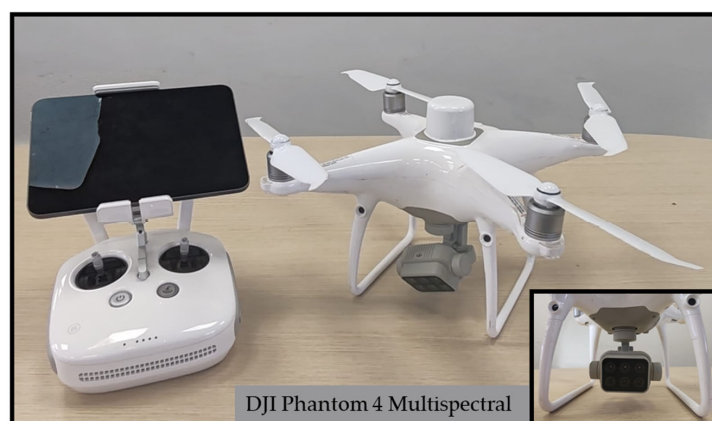
Figure 5. DJI Phantom 4 Multispectral UAV used for remote sensing measurements.
